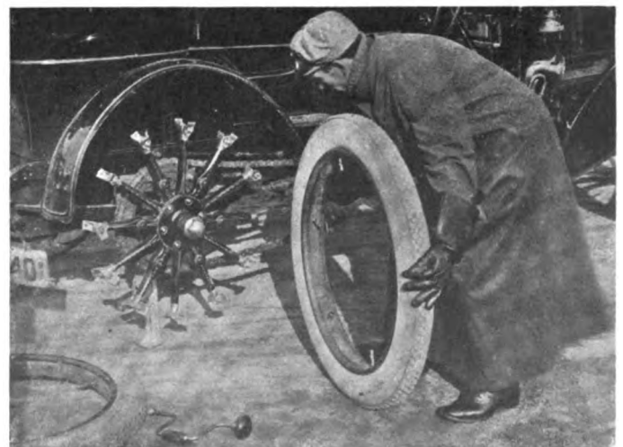
HEAVY DISMOUNTABLE TIRE BEING FIXED ON ITS RIMLESS WHEEL.
